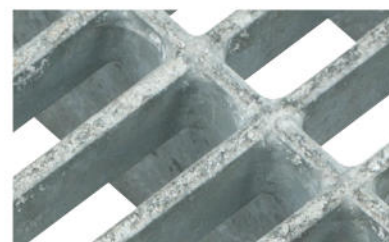
Protective oxidised layer
