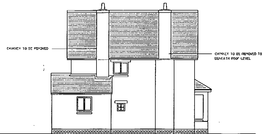
EXISTING NORTH ELEVATION
