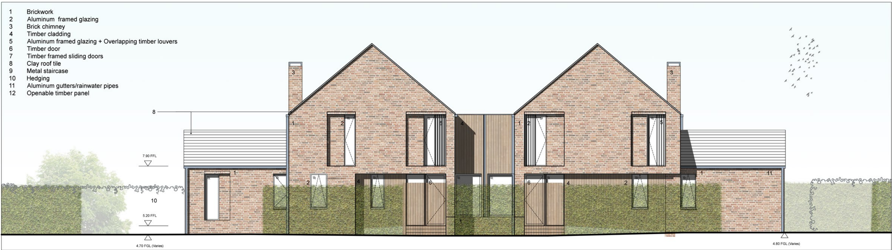
01 PROPOSED SOUTH EAST ELEVATION
