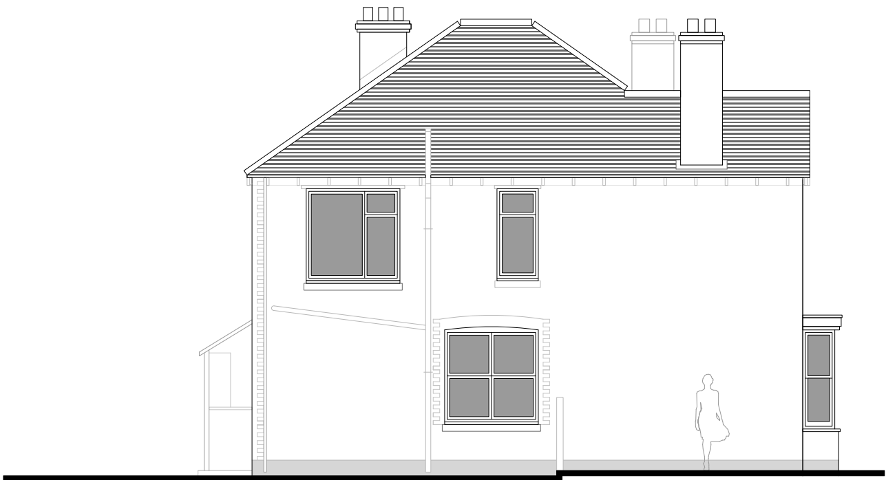
Existing Side Elevation at 1:100 scale SOUTH EAST
