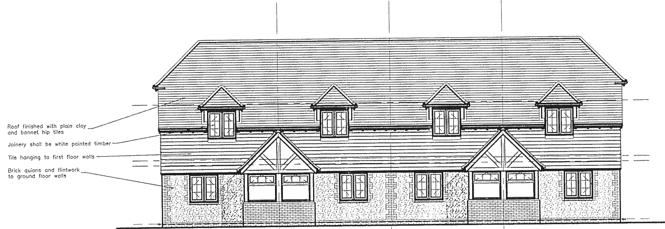
Unit 5 Unit 6 Unit 7 Unit 8 West Elevation
