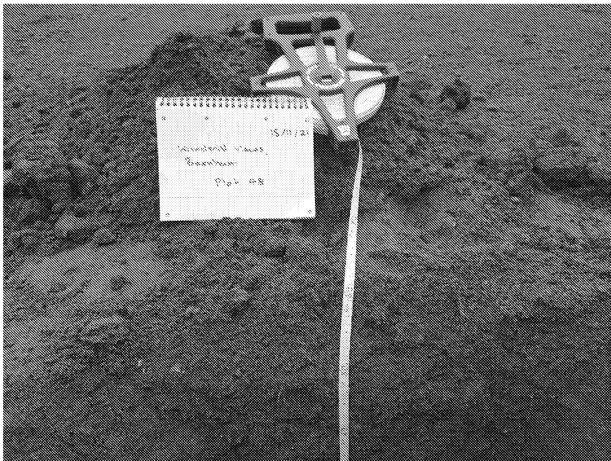
Capping depth – plot 48 (600 mm)
