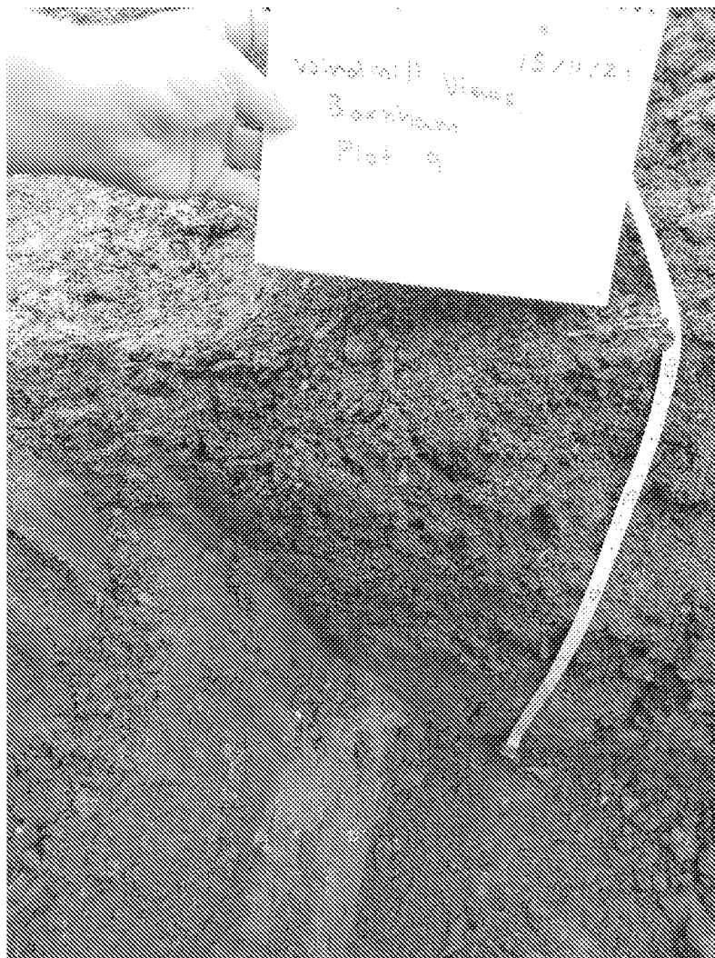
Capping depth – plot 9 (600 mm)
