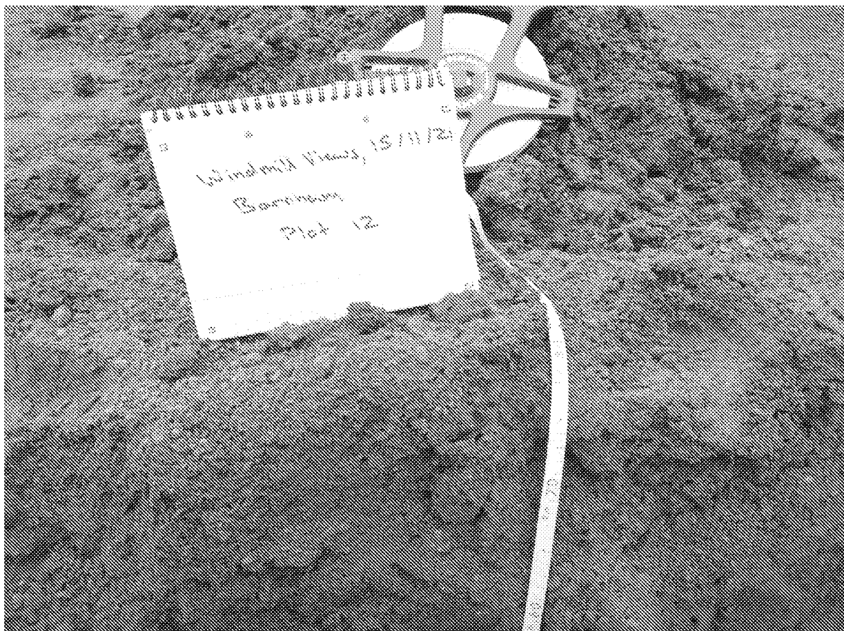
Capping depth – plot 12 (800 mm)
