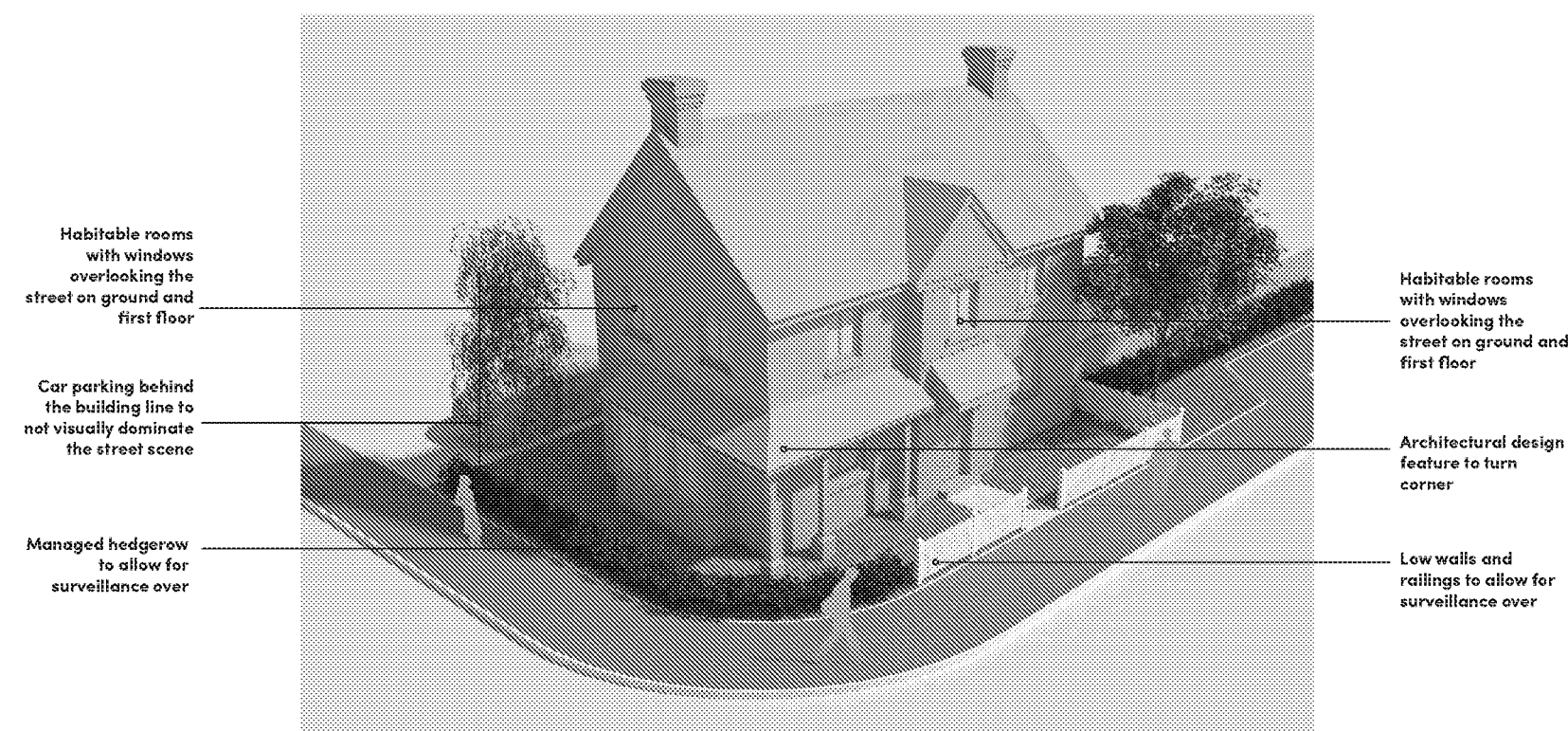
FIGURE 53. Illustration showing how buildings will turn corners
