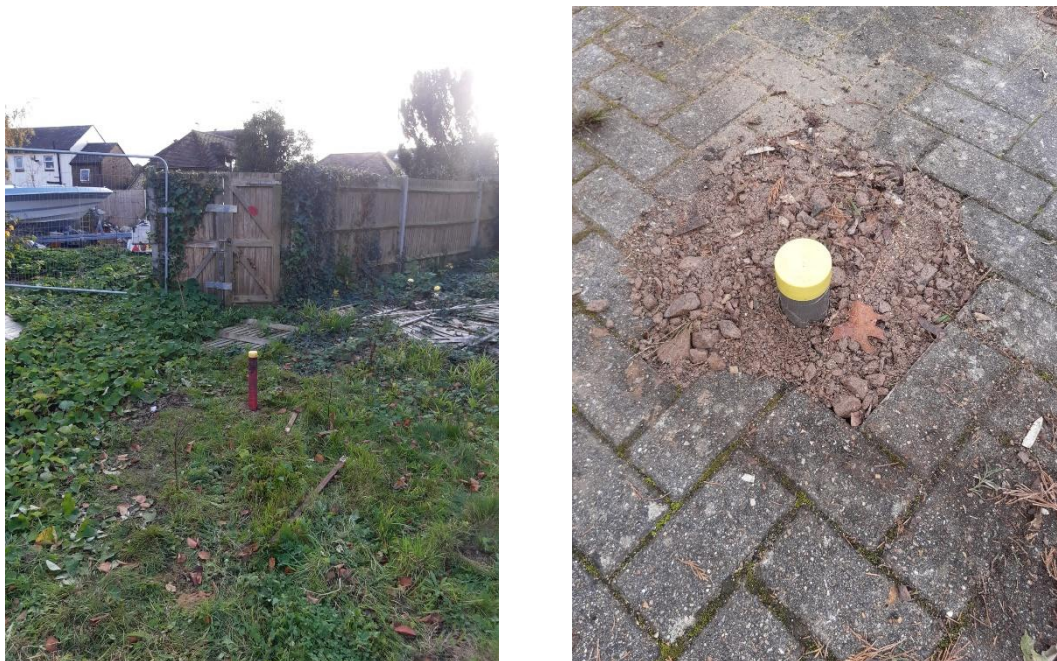
Fig 3. Groundwater Monitoring Well locations
