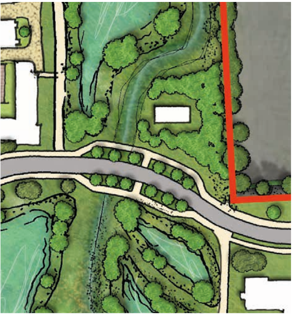
6 North to south pedestrian and cycle crossing of East-West Link Road - an at-grade crossing with a landscape island in the centre of the road
