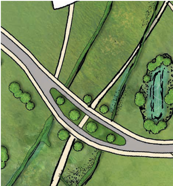
1 North to south pedestrian and cycle crossing of East-West Link Road - an at-grade crossing with a landscape island in the centre of the road
