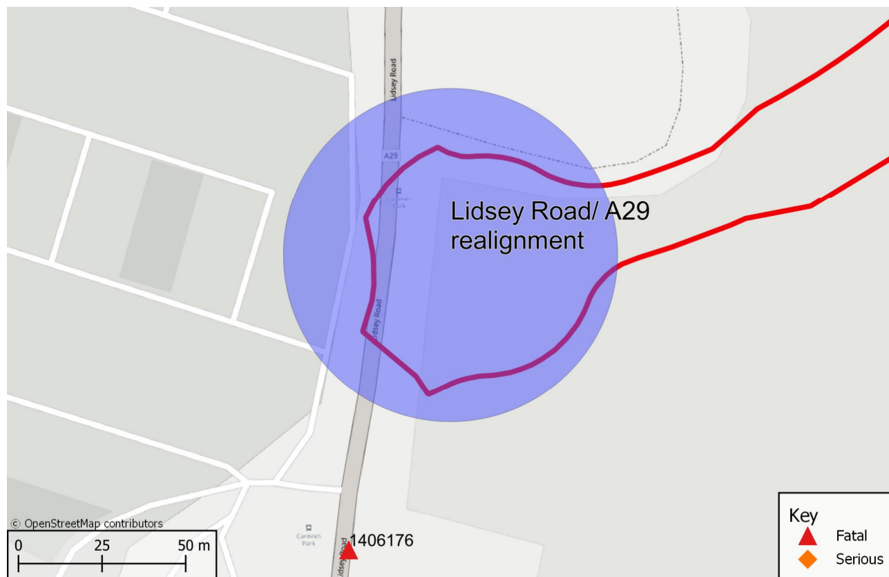
Figure 6: A29 / Lidsey Road alignment
