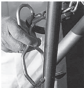
Step 1&2 – Snap the 'lifting hook' onto the SPEL lifting/locating/locking system handle shaft.
