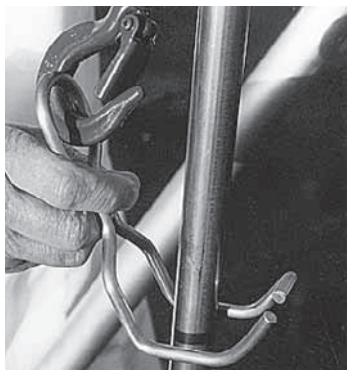
Step 1&2 – Snap the 'lifting hook' onto the SPEL lifting/locating/locking system handle shaft.
