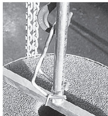
Step 6 – Raise the lifting chain to engage the 'lifting hook' with the lifting hooks on the bottom bracket.
