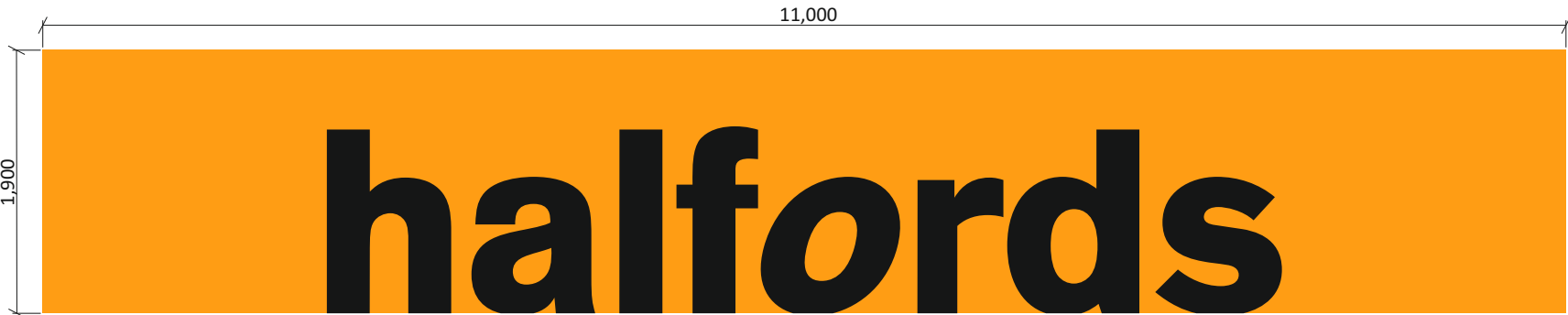
Scale 1:50 11,000 x 1,900mm Replacement flex face skin Retain existing illumination. Paint existing signcase black
