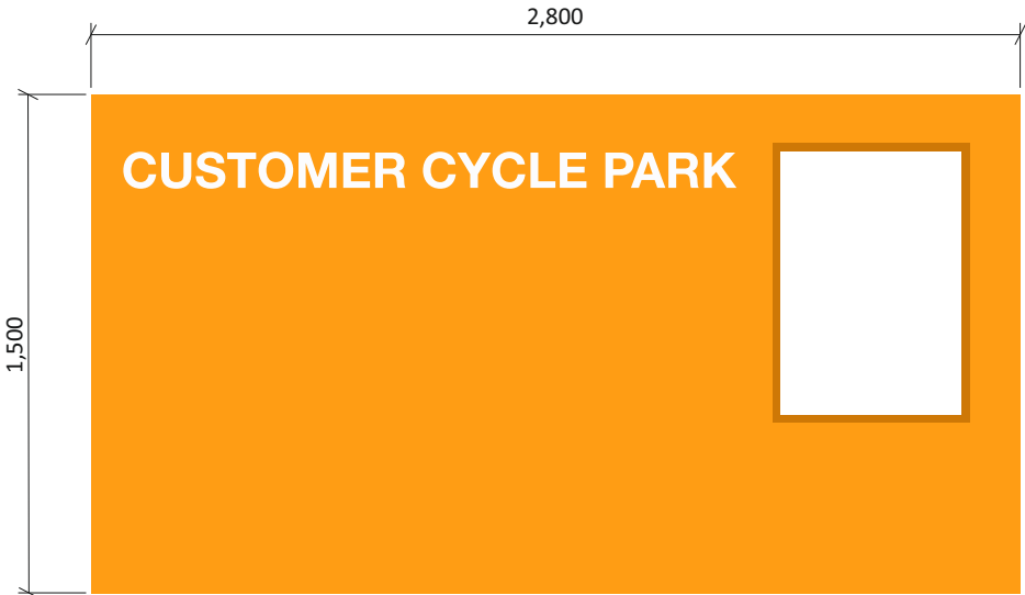
Scale 1:25 CUSTOMER CYCLE PARK Wall mounted 2,800 x 1,500mm aluminium panel c/w with white vinyl to face and A1 Clip frame.
