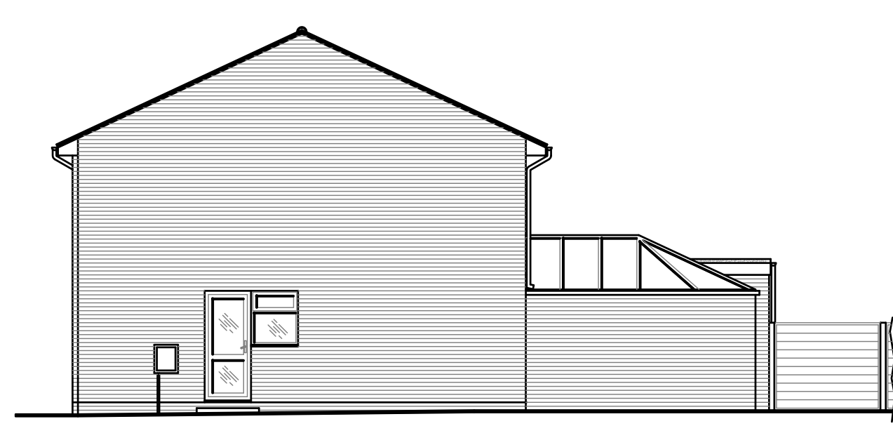
Proposed North Elevation 1/100 Garage Removed
