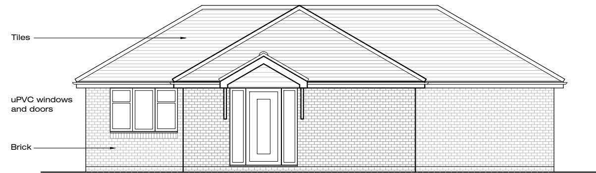
South-West Elevation - As Proposed
