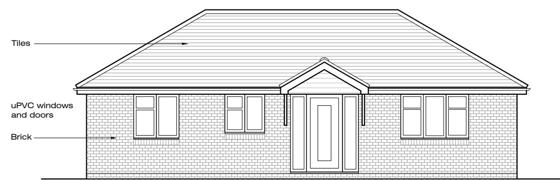
South-East Elevation - As Proposed
