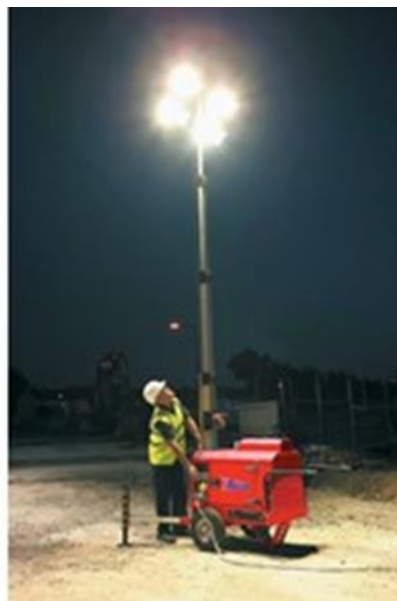
Typical Mobile Lighting Tower
