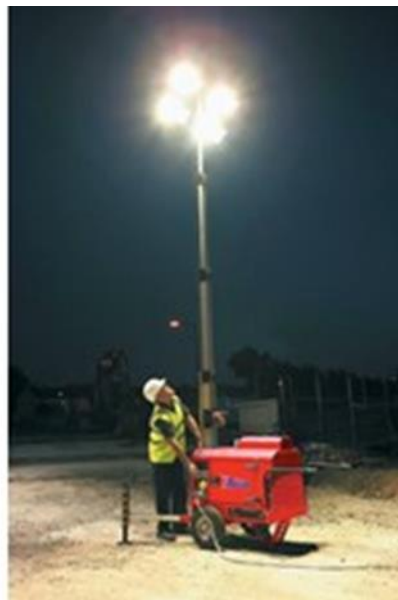
Typical Mobile Lighting Tower
