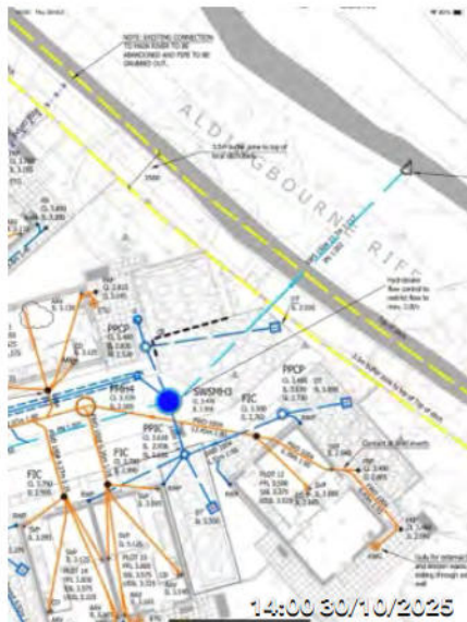
Hydro Break, Flow Control Assigned To Lovells SWSMH3 Storm manhole housing the hydro break.
