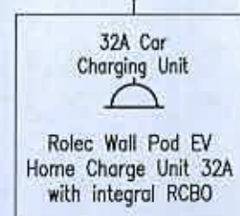
Detached Garage Car Charging Point
