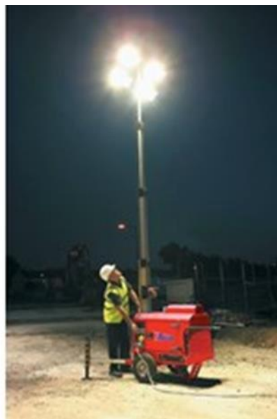
Typical Mobile Lighting Tower
