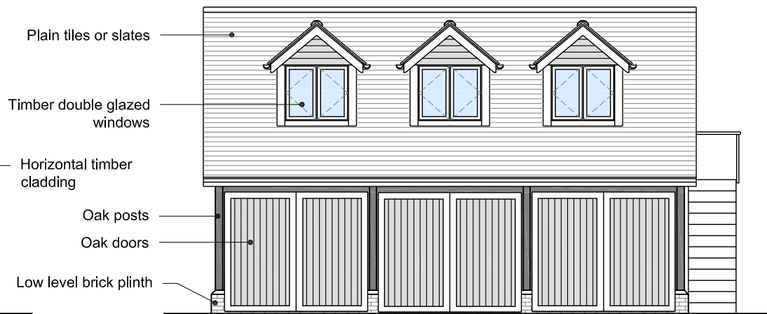
GARAGE FRONT ELEVATION (1:100)
