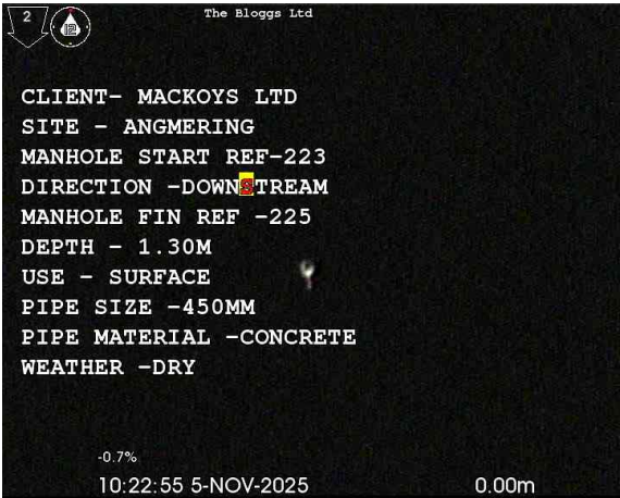
1, 00:00:00, 0.00 m Start node, manhole, reference: 223
