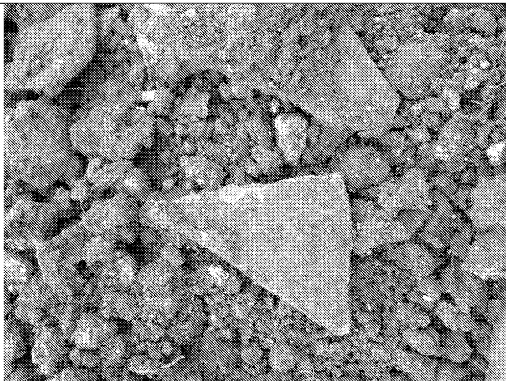
MTP308: Fragment of asbestos (chrysotile) cement.
