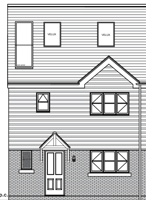
Front Elevation (weather boarding)
