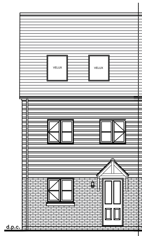
Front Elevation (weatherboarding)
