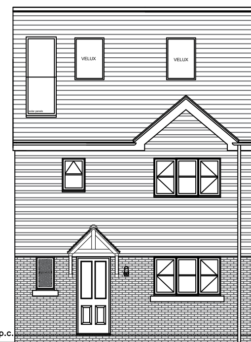
Front Elevation (weather boarding)
