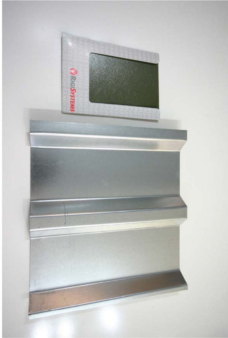
+SM Warehouse elevations - Trapezoidal steel cladding (fir green RAL 6022) - sample to be supplied as part of this submission
