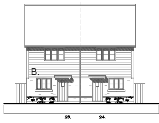
FRONT ELEVATION - West [3 BEDROOM] Semi-detached houses PLOTS 23 & 24
