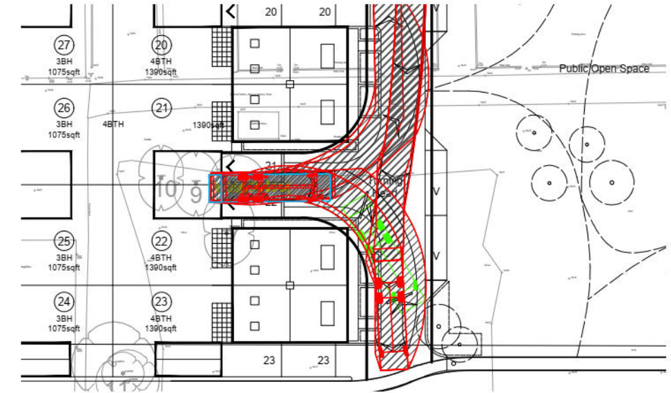
Refuse turning head tracking compliance from Odyssey
