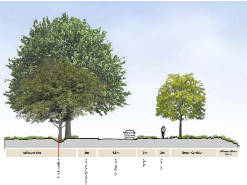
Street section - Western edge of proposed footpath / cycleway within extent of existing hard surfacing
