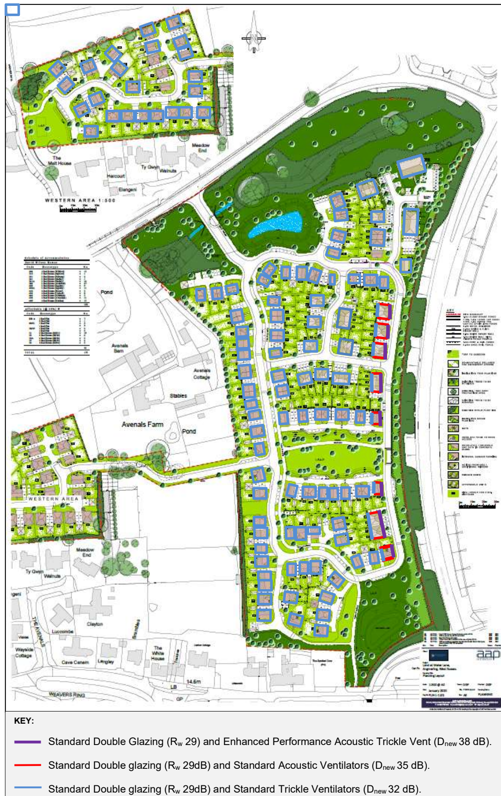
Figure 7.1: Acoustic Performance Recommendations
