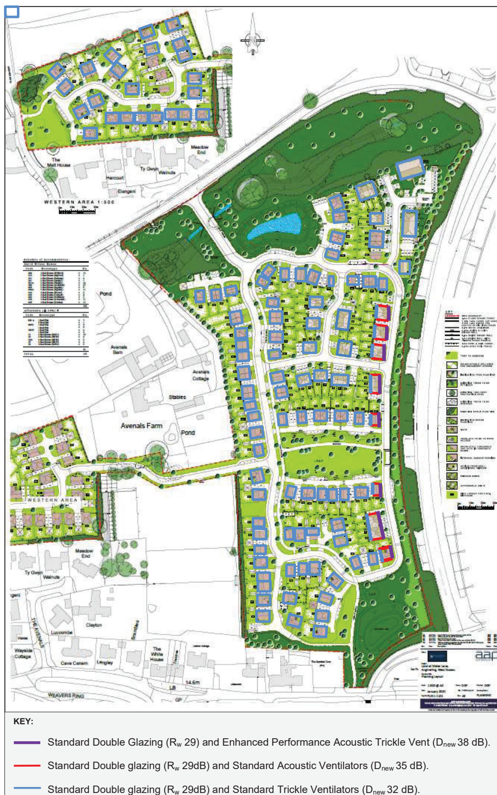
Figure 7.1: Acoustic Performance Recommendations
