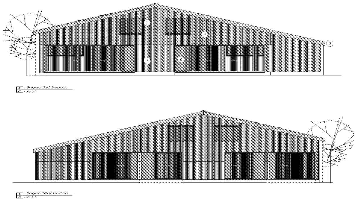
Figure 2- Roller batten doors (East and West Elevations)
