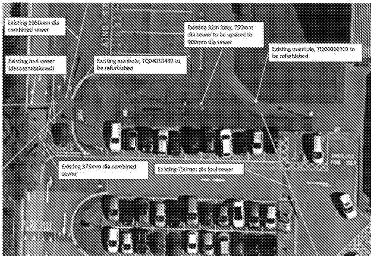
Photograph 08 – Proposed works within the car park of Littlehampton Swimming and Sports Centre
