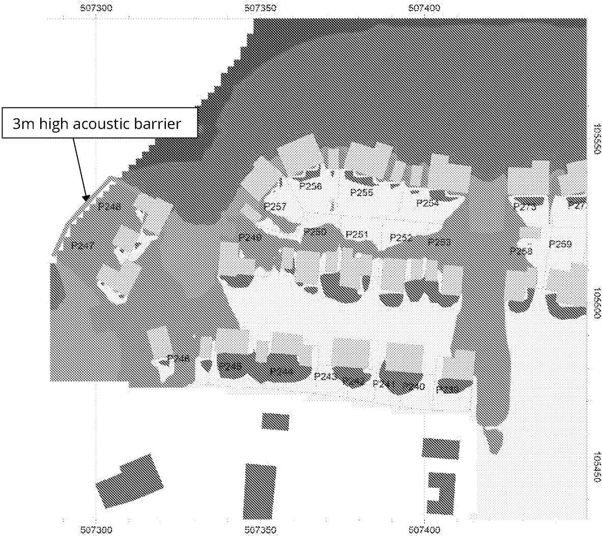
Figure C3: Daytime Noise Contours with 3m Acoustic Barrier
