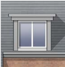
Flat roof dormer windows
