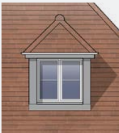
Pitched roof dormer windows
