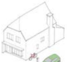
Bicycle storage closer to the house than vehicle parking. Electric charging points for cars.
