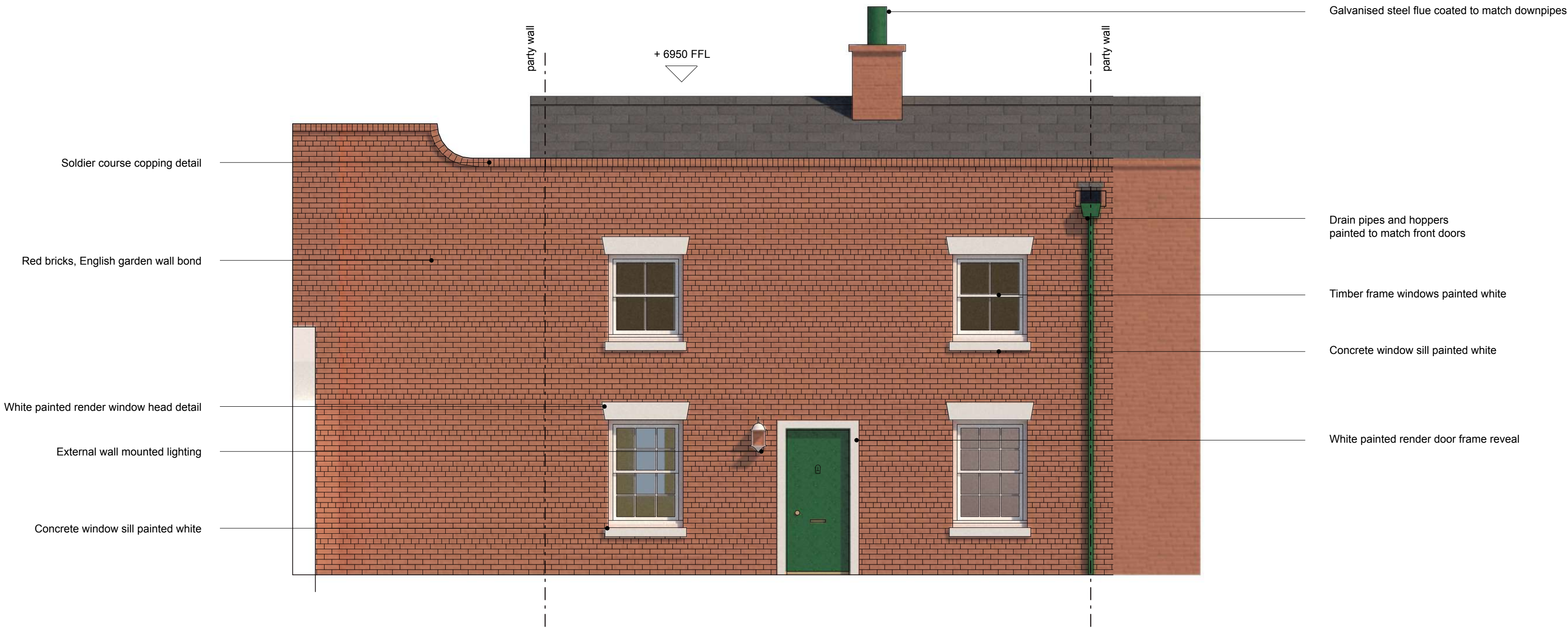
A Terrace A (3 bed) - Front elevation (North)
