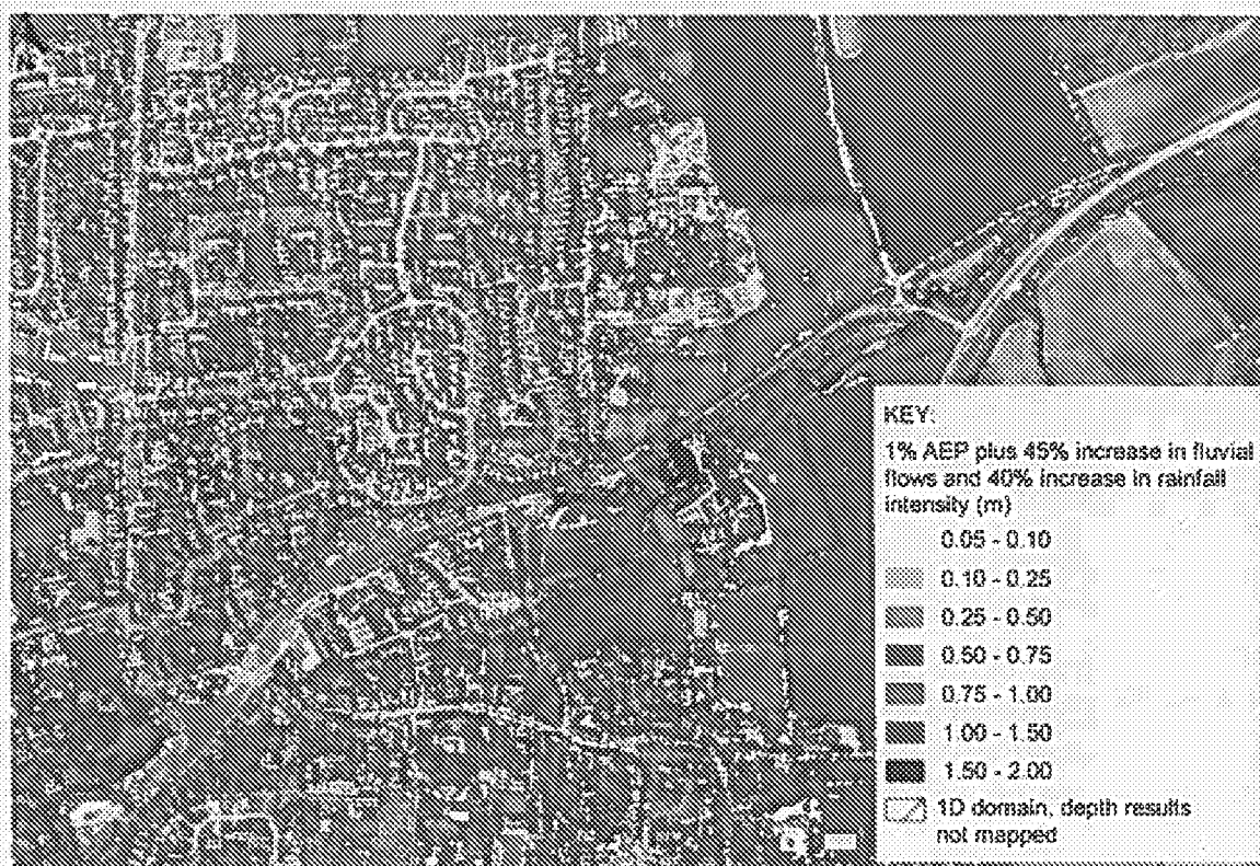
Figure 7.2: Baseline flood risk to Angmering from a 1% AEP + 45%cc event
