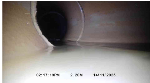
2, 00:00:13, 2.20 m Finish node, major connection without manhole, reference: MAIN
