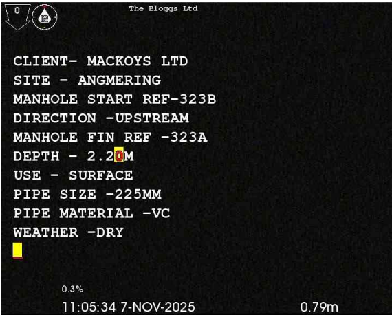
1, 00:00:00, 0.00 m Start node, manhole, reference: 32B
