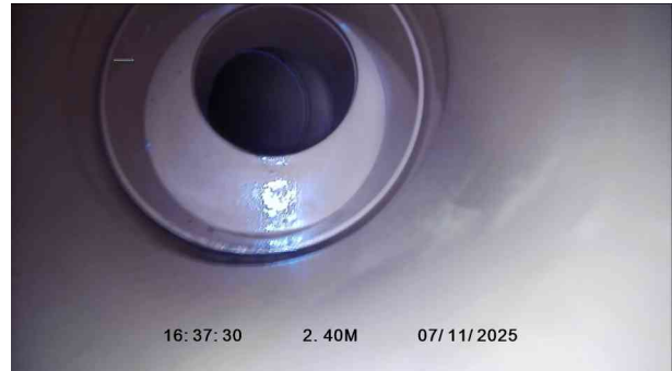
2, 00:00:28, 2.40 m Pipe size changes, new size(s), 100mm high
