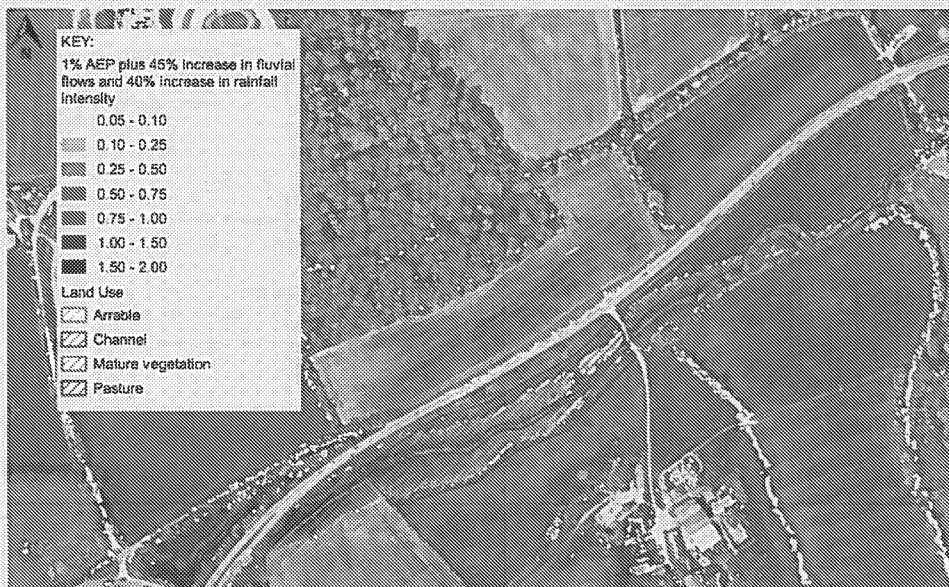
Figure 8.10: Overlay of peak flood attenuation extent on agricultural land with breakdown by arable / grazing land areas.
