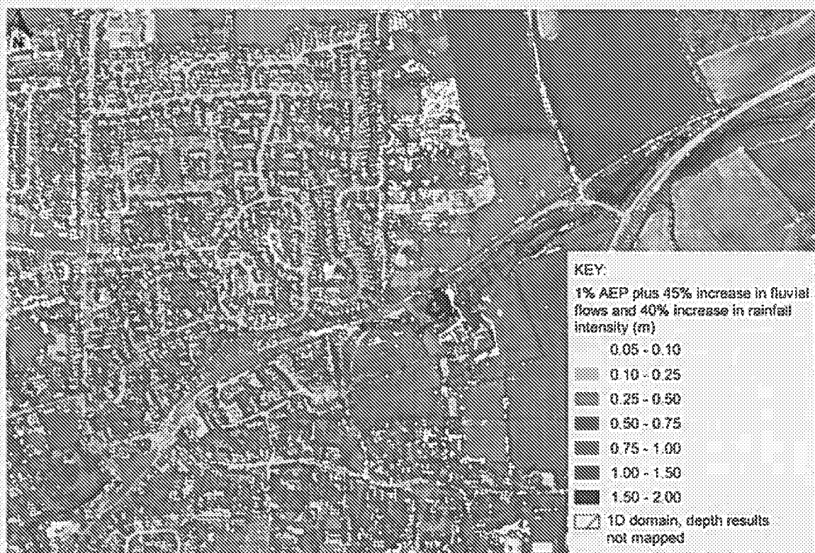
Figure 8.1: FAS flood risk to Angmering from a 1% AEP + 45% cc event
