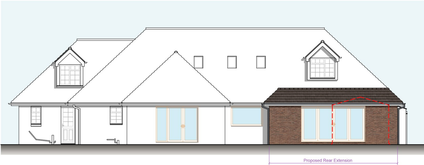
East Elevation (Rear) – 1:100
