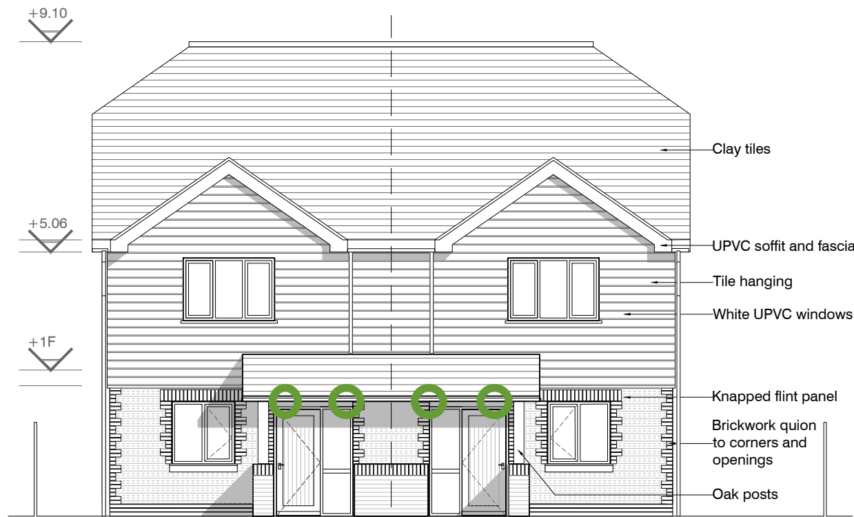
Front Elevation (West)
