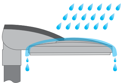
1. "Free draining" curved heat sink eliminates ponding of fluids
