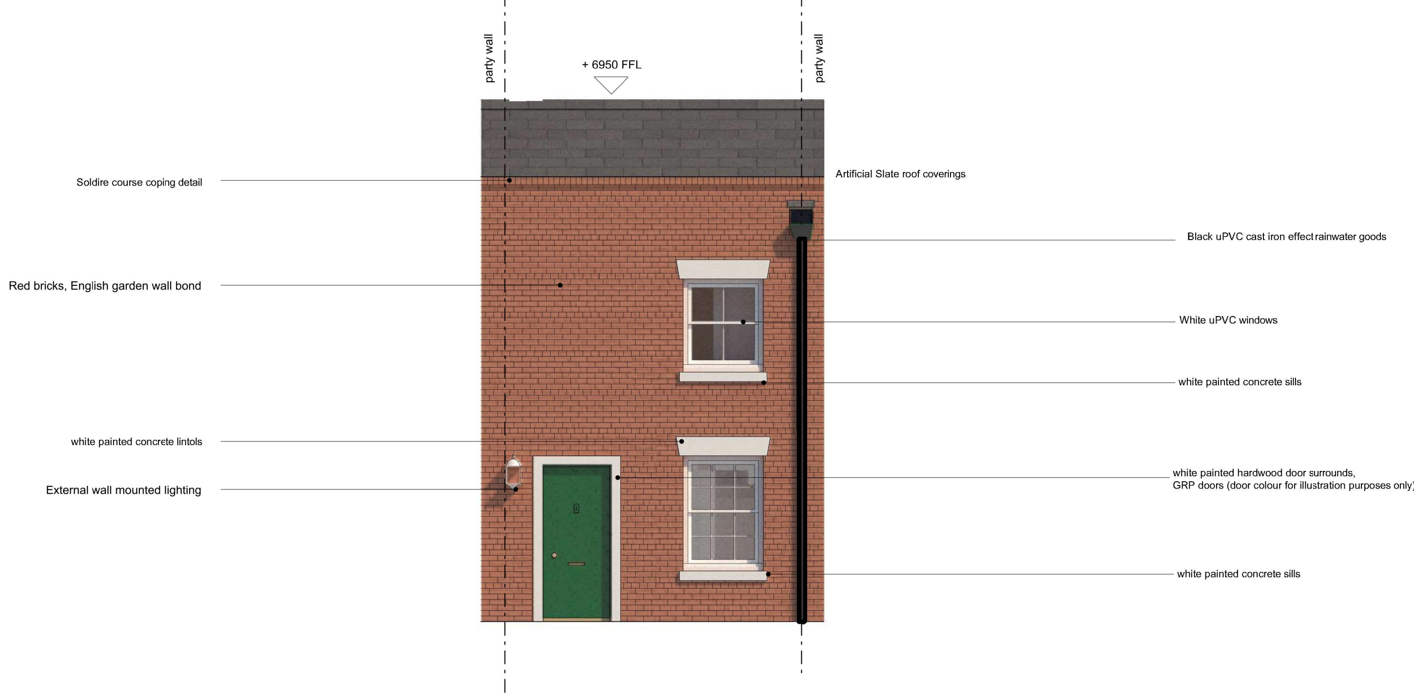
A Terrace A (1 bed) - Front elevation (North)
