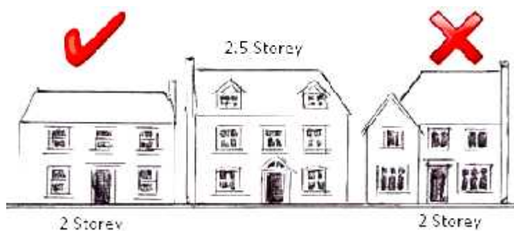
Fig 6.5: Example of Acceptable and unacceptable 2 storey heights
