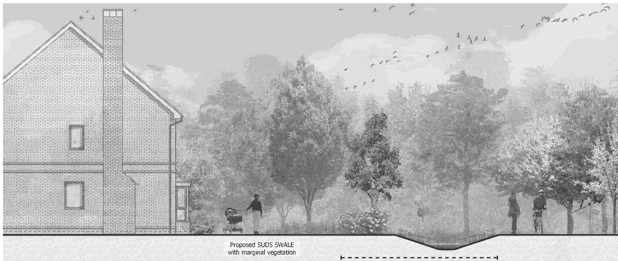
ILLUSTRATIVE CROSS SECTION THROUGH THE SWALE WHEN PERIODICALLY WET
