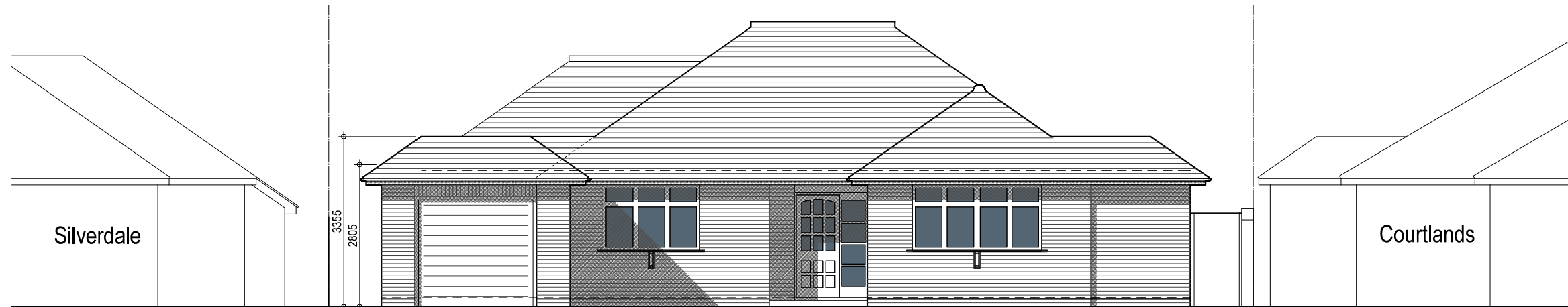
Front (East) Elevation This wall rendered and painted
