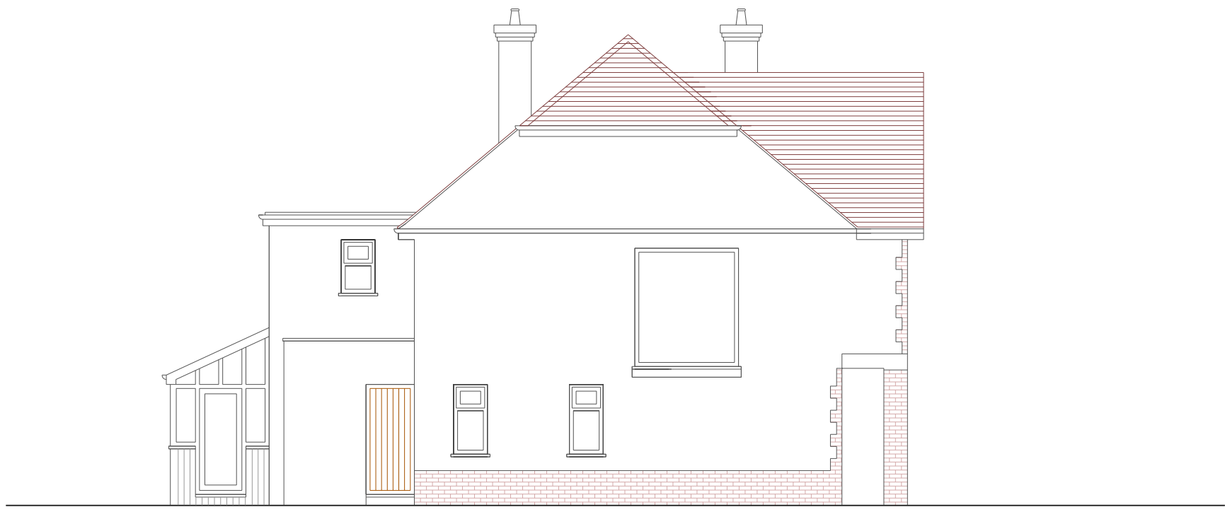
EXISTING SIDE ELEVATION
