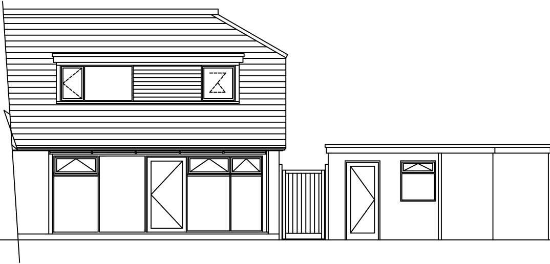
Existing West Elevation
