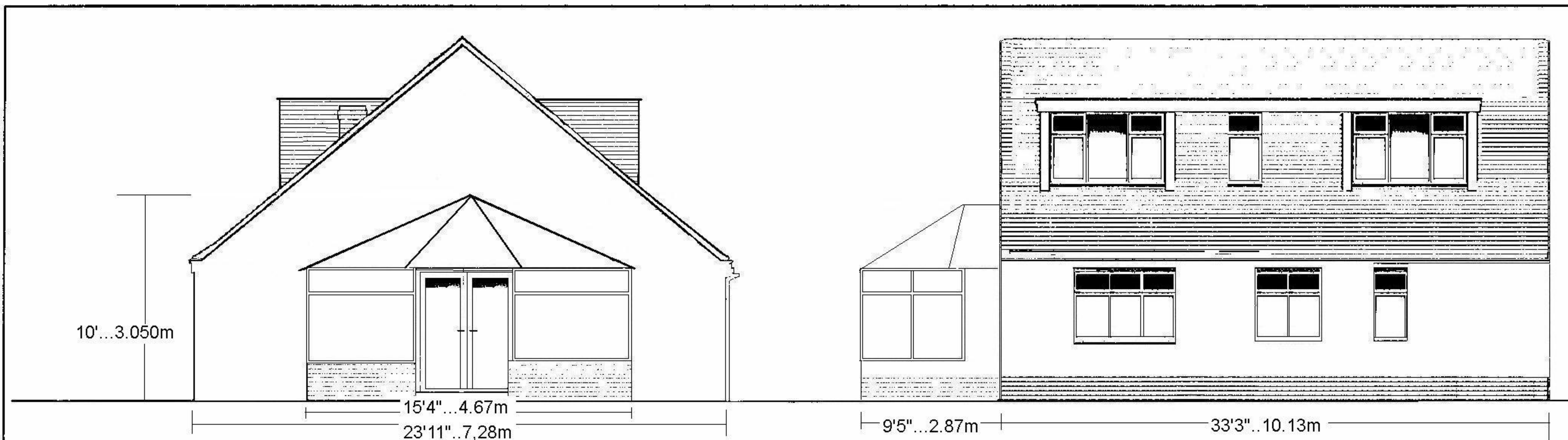
Side and front Elevations
